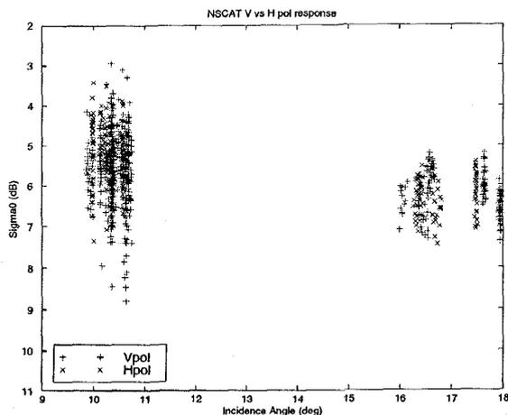
Figure 2: NSCAT dual-polarization  $\sigma^0$  measurements for incidence angles less than  $18^\circ$  over the study region from JD 25-55, 1997.
