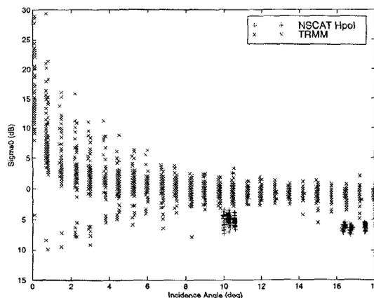
Figure 3: Comparison of TRMM and NSCAT H-pol  $\sigma^0$  measurements over the study region. TRMM data is from days Feb. 24-25, 1998 while NSCAT data is from JD 25-55, 1997.
