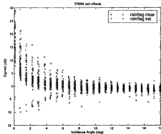
Figure 5: Comparison of rain flagged TRMM surface  $\sigma^0$  measurements over the study region during Feb. 24-25, 1998.
