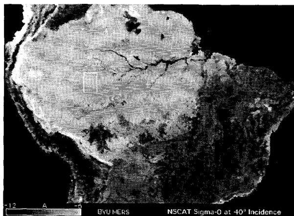
**Figure 1:** NSCAT SIRF  $\mathcal{A}$  image ( $\sigma^0$  at 40° incidence angle) of the Amazon from two weeks of data in 1997. The study region is outlined.
