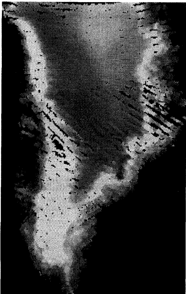
Figure 1. An \mathcal{A} image generated using vertically-polarized \sigma^0 measurements made during the last month of the SASS mission.
