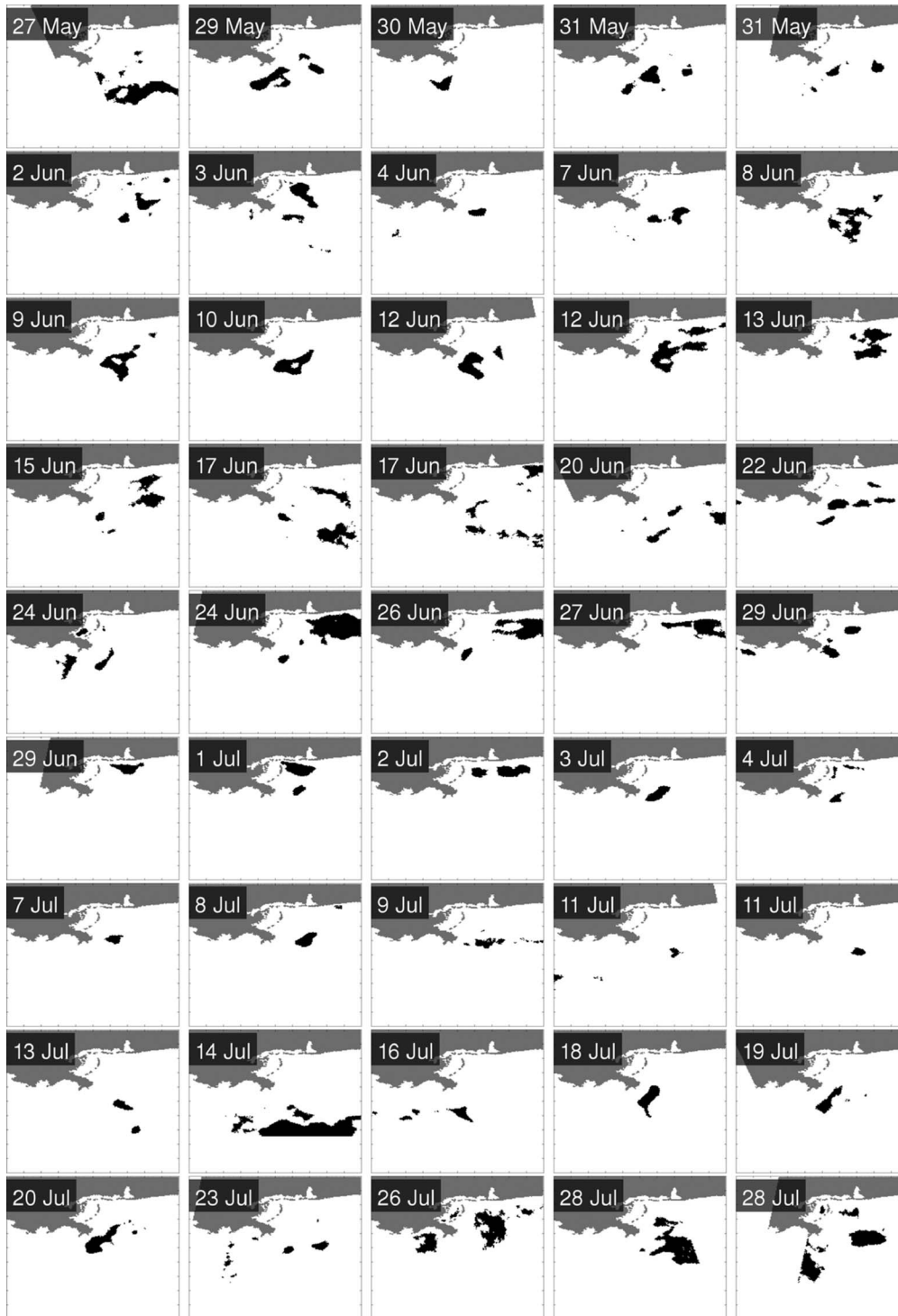
Fig. 10. Selected time series of mapped oil. Each image is the thresholded backscatter error for the date indicated in the upper left corner. The ASCAT pass may not completely cover the region on a given day, leading to a diagonal crop in some of the images.
