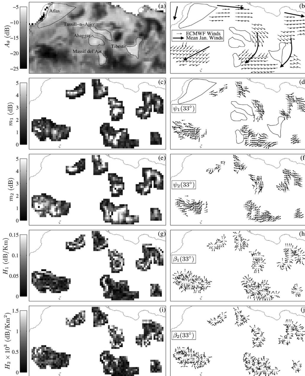
Fig. 11. Spatial maps of the model parameters at  $\theta = 33^\circ$  from NSCAT data during JD 1–30, 1997, for Saharan ergs. (a)  $A_\theta$ , (c)  $m_1$ , (d)  $\psi_1$ , (e)  $m_2$ , (f)  $\psi_2$ , (g)  $H_1$ , (h)  $\beta_1$ , (i)  $H_2$ , and (j)  $\beta_2$ . (b) Average wind behavior over the ergs during January (JD 1–30), 1997.
