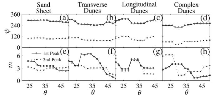
Fig. 10. (a)–(d)  $\psi$  as a function of  $\theta$  showing both  $\psi_1$  and  $\psi_2$  over the four sand surface types at locations 16, 5, 10, and 18. (e)–(h) Similar plots of  $m$  as a function of  $\theta$  showing both  $m_1$  and  $m_2$ .
