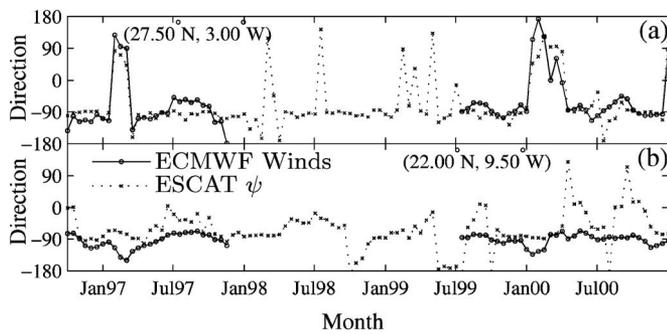
Fig. 15. Comparison of the long-term temporal behavior of ECMWF mean wind directions and  $\psi$  orientations derived from ESCAT data at two locations.
