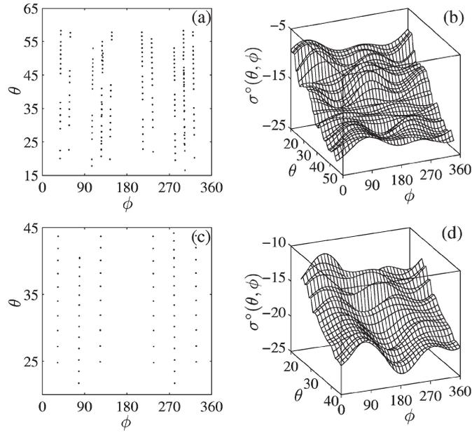
Fig. 4. (a) and (c) Plots of  $\theta$  and  $\phi$  for each measurement during JD 1–30, 1997, at location 18 from NSCAT and ESCAT, respectively. (b) and (d)  $\sigma^\circ(\theta, \phi)$  model surface fits as a function of  $\theta$  and  $\phi$  from NSCAT and ESCAT, respectively. The rms errors of model fits for NSCAT and ESCAT are 3.63 and 2.97 dB, respectively.
