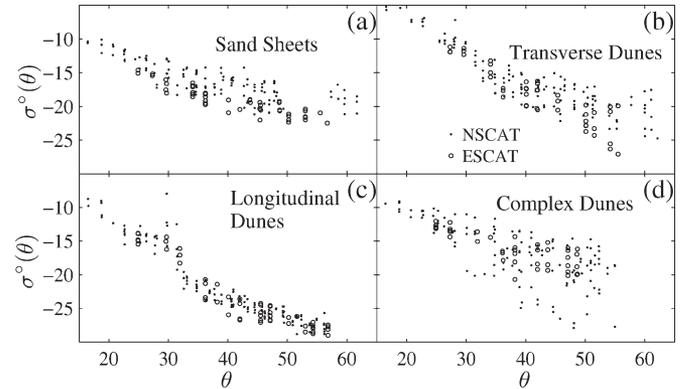
Fig. 3. NSCAT and ESCAT  $\sigma^{\circ}(\theta)$  at  $\phi = 127^{\circ}$  during JD 1–31, 1997, for (a) sand sheets, (b) transverse dunes, (c) longitudinal dunes, and (d) complex dunes corresponding to locations 5, 10, 16, and 18.
