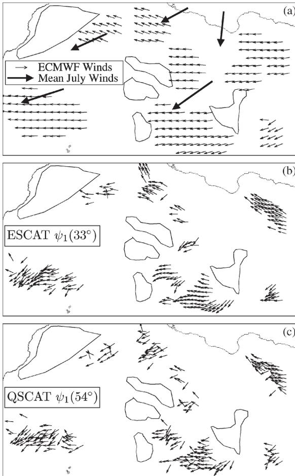
Fig. 12. (a) Average wind map JD 182–212, 1997, (b)  $\psi_1$  computed for ESCAT data corresponding to (a), and (c)  $\psi_1$  computed for QSCAT data during JD 182–212, 2000.
