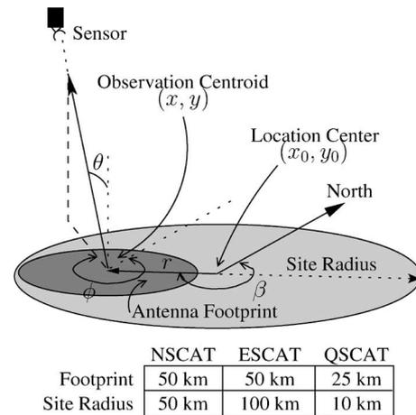
Fig. 1.  $\sigma^\circ$  observation geometry parameters for a single resolution element within a circular area centered at  $(x_0, y_0)$ . The footprint size and site radius are listed for each sensor.
