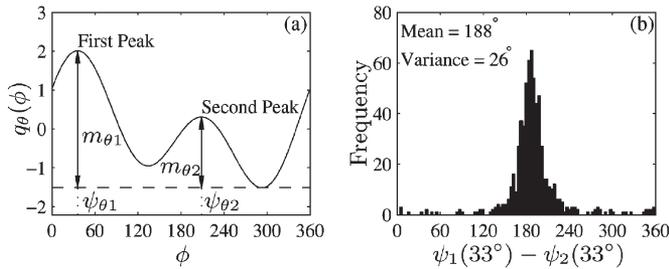
Fig. 9. (a) Slice through  $q_\theta(\phi)$  surface fit is shown to define azimuth angle of a peak ( $\psi$ ) and magnitude ( $m$ ) of  $\phi$ -modulation at  $\psi$ . (b) Histogram of angular difference between two peaks over all the ergs showing that, in general, two peaks of  $\phi$ -modulation are separated by  $180^\circ$ .
