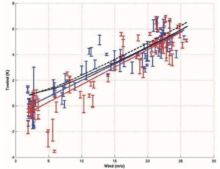
Fig. 6. Measured wind speed dependence for (blue) 3R antenna and (red) 2L antenna. The model results obtained with twice the Durden and Vesecky model spectrum are superimposed (black line). (Dashed line) At incidence  $21.5^\circ$ . (Solid line) At incidence  $38.4^\circ$ .
