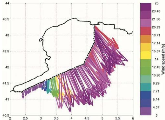
Fig. 4. High-resolution wind speed retrieved from QSCAT measurements along the plane track (dashed line).
