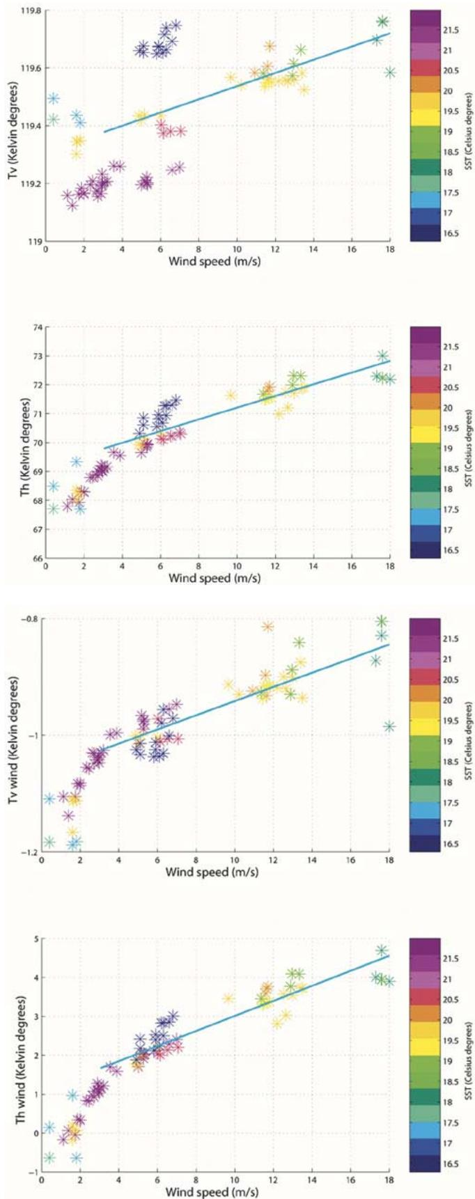
Fig. 8. Wind speed dependence in (top) vertical and (bottom) horizontal polarizations measured at  $44^\circ$  incidence angle during WISE 2001 of brightness temperature and  $T_{b\text{wind}}$ .
