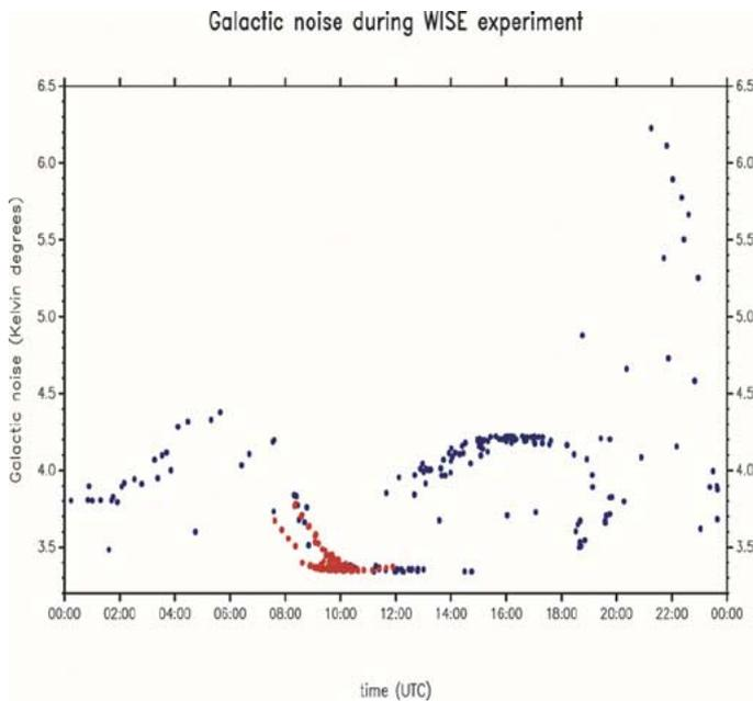
Fig. 9. Galactic noise seen by the radiometer during measurements at (red) incidence  $44^\circ$  and (blue) at  $45^\circ$  (blue).
