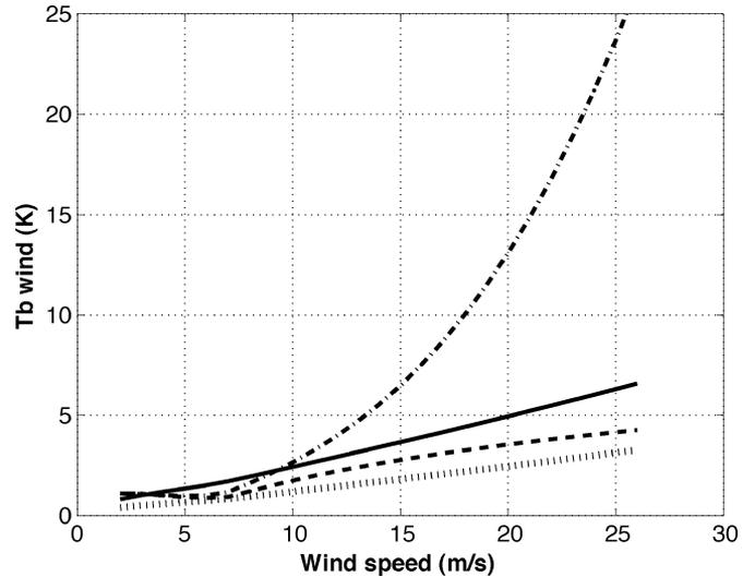
Fig. 7. Modeled wind speed dependence using different spectral parameterizations: (Dotted line) Durden and Vesecky, (dashed line) Elfouhaily, (solid line) twice Durden and Vesecky, (dashed-dotted line) Elfouhaily plus foam.
