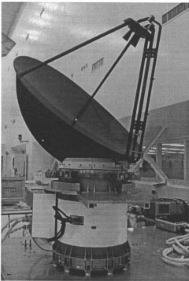
Fig. 2. SeaWinds antenna and rotary mechanism.
